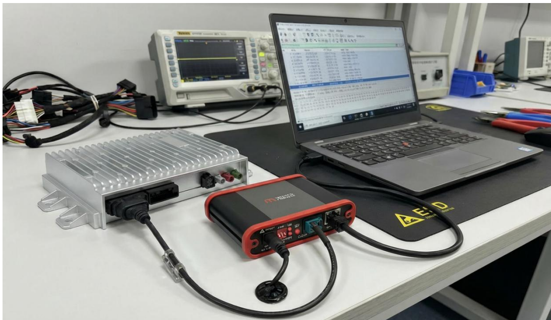
Scenario 1: Laboratory ECU Communication Debugging
